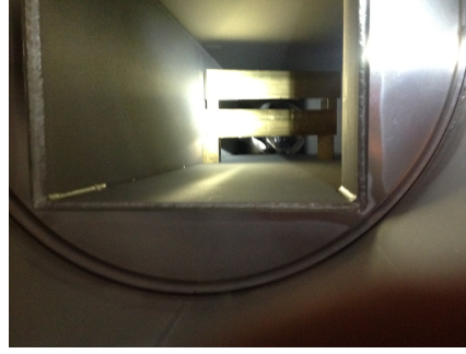
Figure 8: Photo of the brass collimator placed in the center of the bending magnet ASK51. The electrons that are deflected by the electrostatic separator stop in the brass.
