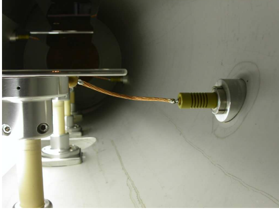
Figure 4: Left: Inside the beampipe: copper connector between the deflector plate and the feed-through. Right: Over-current protection circuit connected and installed in a MOSFET stack.
