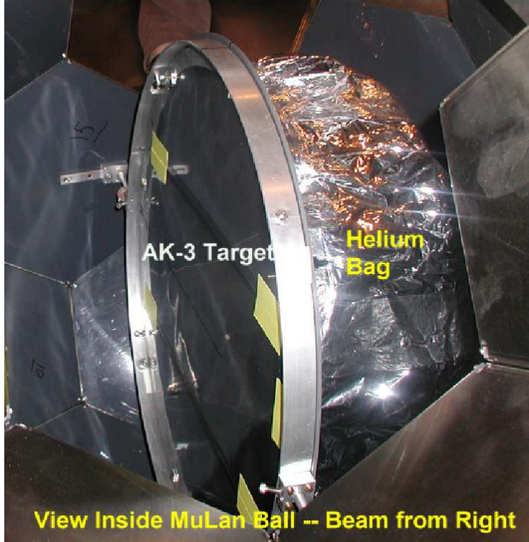
Figure 7: View inside the MuLan ball of the new target assembly and helium bag. The target is a large sheet of AK-3 and, in this photo, the helium bag is not fully inflated. The beam enters from the right.
