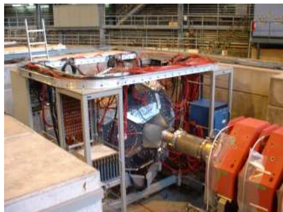
Figure 1: Photograph of \mu Lan detector installed in the \pi E3 beamline.
