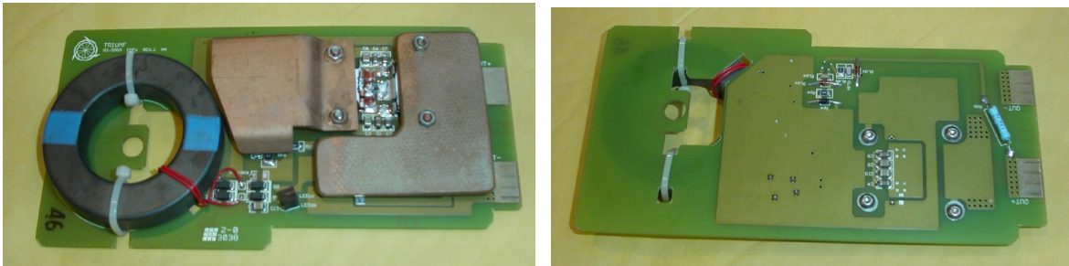
Figure 3: Front and back sides of one MOSFET card. On the front side, one sees the ferrite, the copper shielding of the MOSFET and other electronic parts. Of particular interest is the small resistor located on position C13 (lower middle part). On the back side, one sees clearly the long blue resistor, as well as the drain (OUT +) and source (OUT -) pads.
