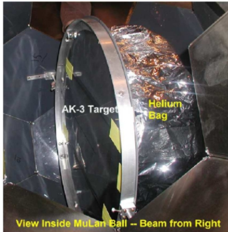
Figure 2. The installed MuLan setup: The helium bag and the AK3 target mounted in the detector center.
